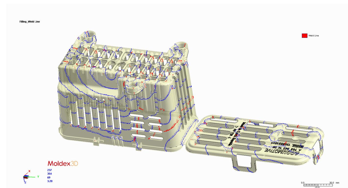
→ The red lines indicate possible weld lines on the part.
